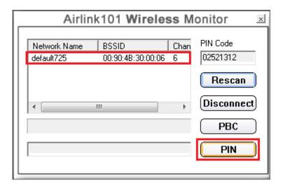
The progress of the WPS connection will be shown in the status bar to tell you that it is successful or failed. If it is failed, verify that you type in the correct PIN code in the Router's configuration page and click the **PIN** button to try again.
